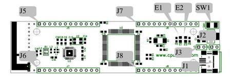
When the StickOS is running the "heartbeat" LED E1 will blink slowly; when the BASIC program in the MCU is running, the "heartbeat" LED E1 will blink quickly. LED E2 may be user controlled on digital output pin "e2".
