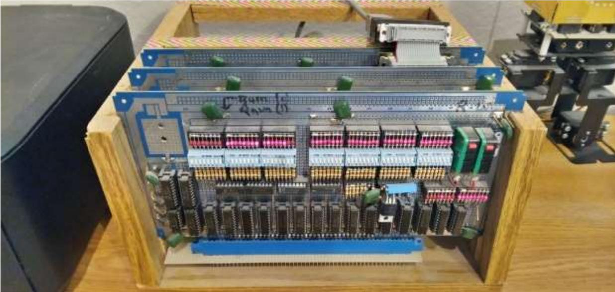
In 1987, the thing powered on and worked on the first try, with maybe 2000 (?) wire wrap connections!
