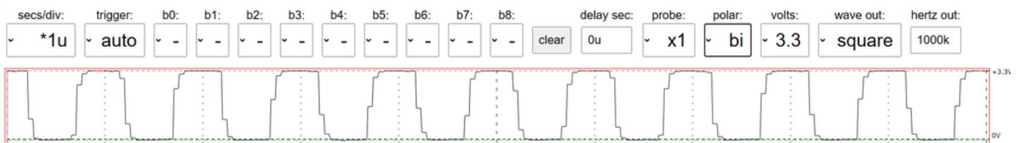
Pushing further to 4 MHz, we see we are still well above the -3db (70.7%) "analog bandwidth" cutoff typically quoted for oscilloscopes, but, Nyquist is now limiting our signal fidelity:
