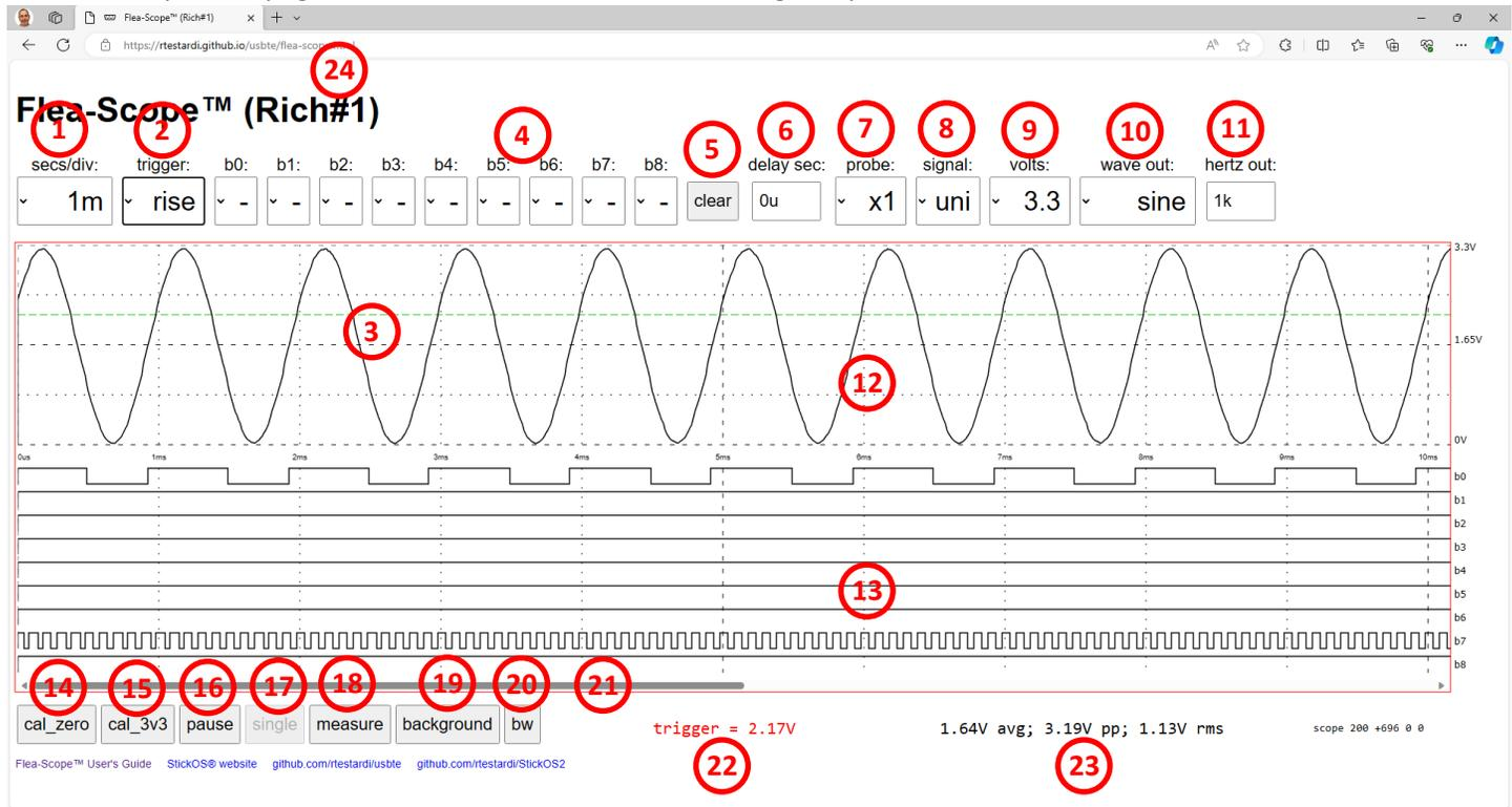
1. horizontal scale selection (secs/div) -- sets sample rate for input capture from 0.5us to 100ms per division
