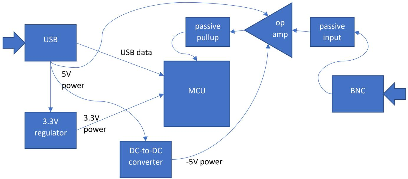
1. USB connector -- supplies 5V power and USB data connectivity to Flea-Scope board
